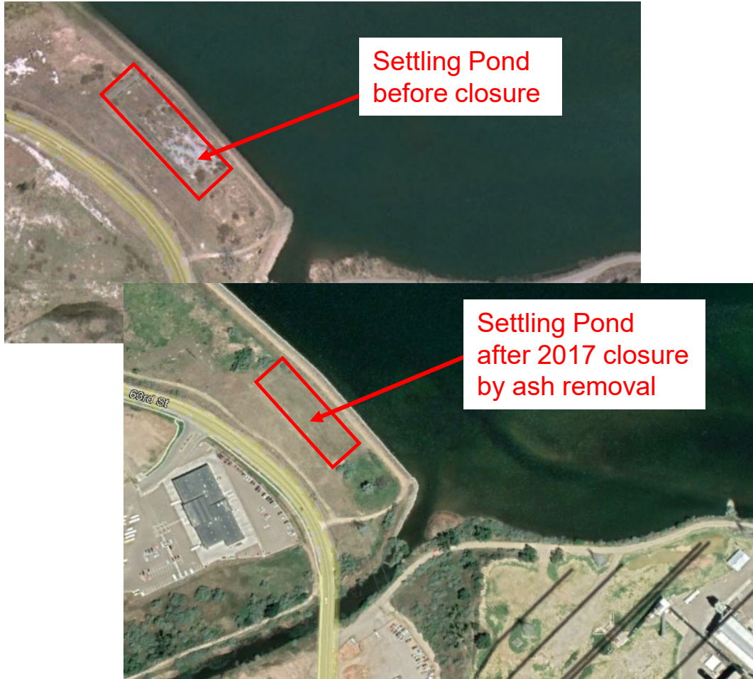
Groundwater Standards Met in 2021 = Clean Closure
